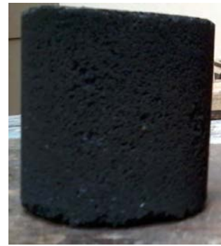
Fig. 1 Specimen of UFS prepared for compression strength.
